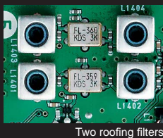
Two roofing filters
